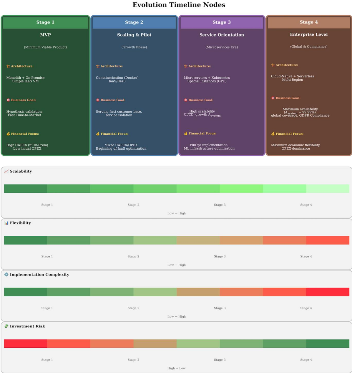
Fig. 4. Stages of architectural evolution of a voice identification system from MVP to enterprise level
